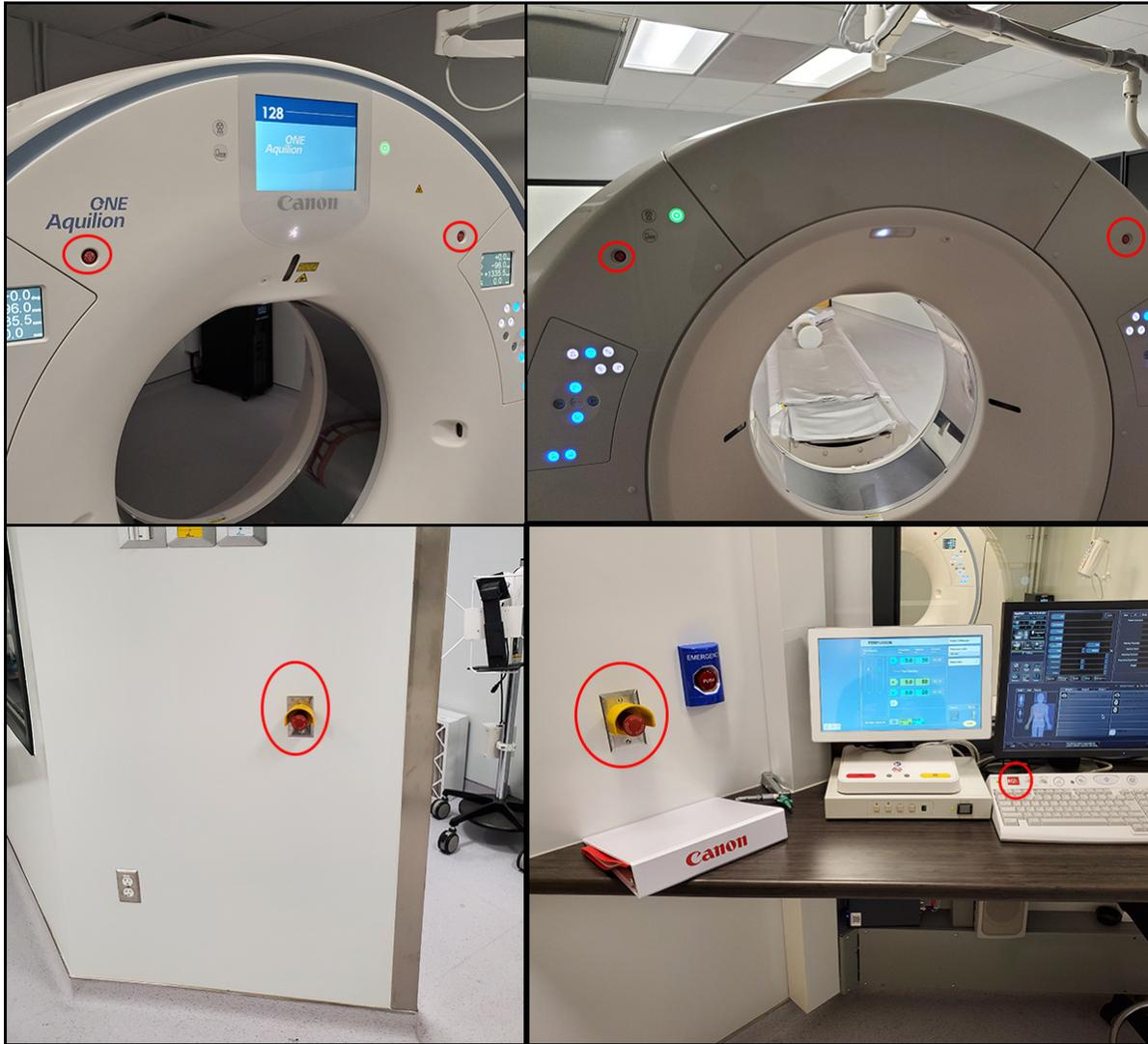
Figure 1: Emergency Stop buttons located on the gantry, on the walls of the operators' console, and on the S-con keyboard.
